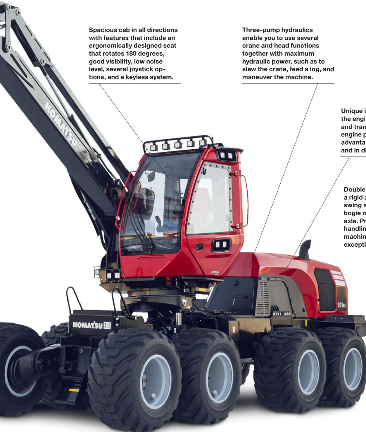
Spacious cab in all directions with features that include an ergonomically designed seat that rotates 180 degrees, good visibility, low noise level, several joystick options, and a keyless system.
