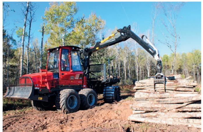
**Larry Poquette operating the new Komatsu 855.1 forwarder equipped with the Comfort Ride hydraulic cab suspension system.**
