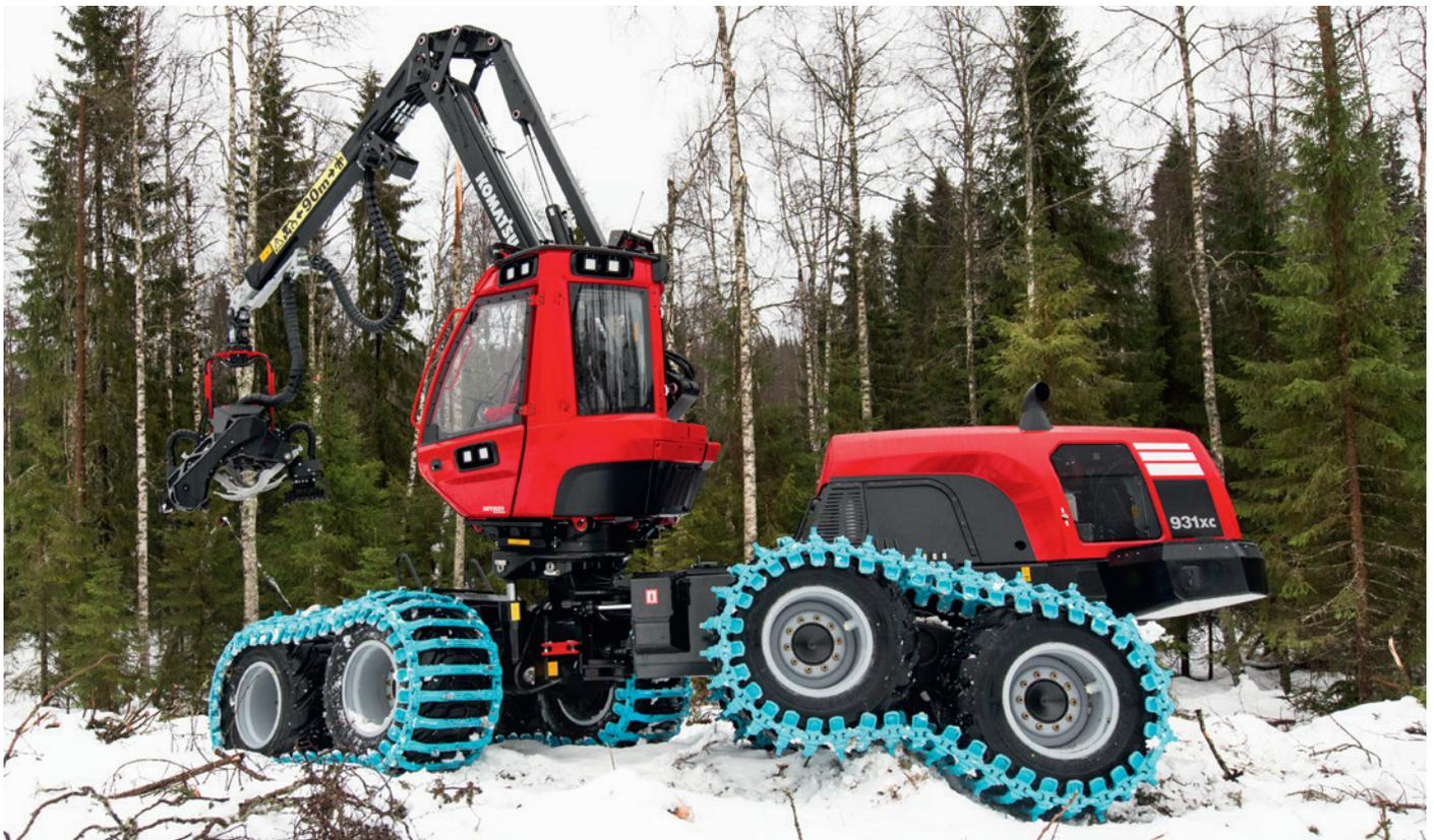
Double suspension entails a rigid articulated joint and swing axle combined with a bogie mounted on the swing axle. Provides maximum mobility and comfort on steep inclines and soft ground.
