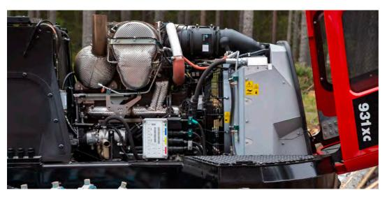
New engine installation compliant with the latest emission legislation. This brings with it a number of benefits, such as a brandnew DEF system, a new exhaust system, and hydraulic valve lifters.
